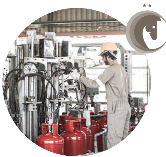
EMGAS Cylinder filling operation
